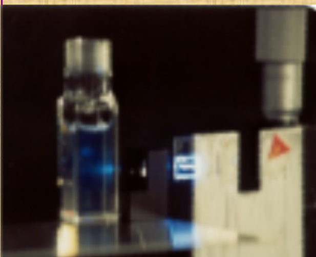
FIG. 2. Lasing action from a nano-structured ZnO thin film
